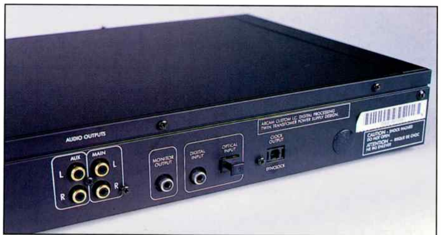
The sync-lock signal is optically coupled to the transport through a glass fibre Toslink; it is identified as Clock Output, at right.
