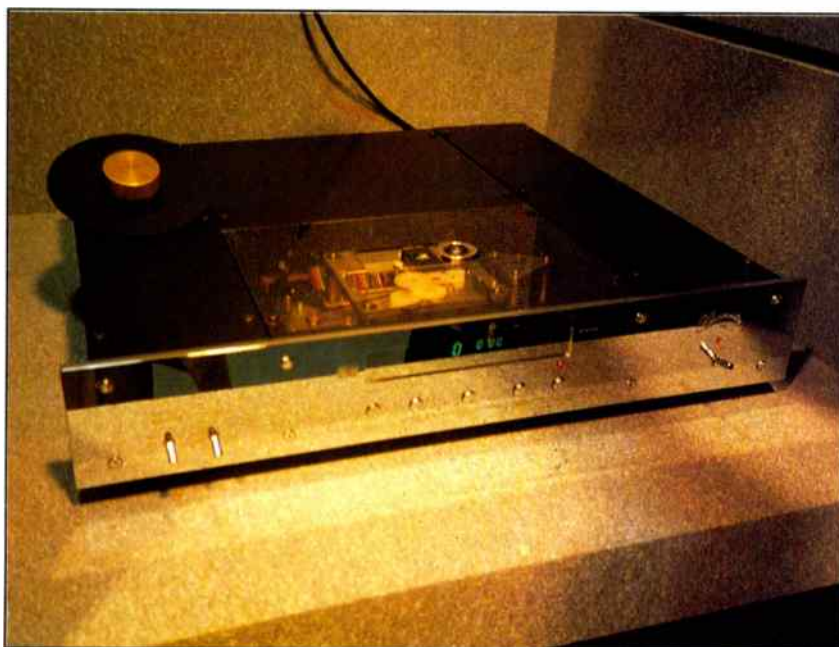
Right: Belt drive reaches Compact Disc in the Burmester 916 transport. It is a top loader: a stabilising disc can be seen in the far left corner.
