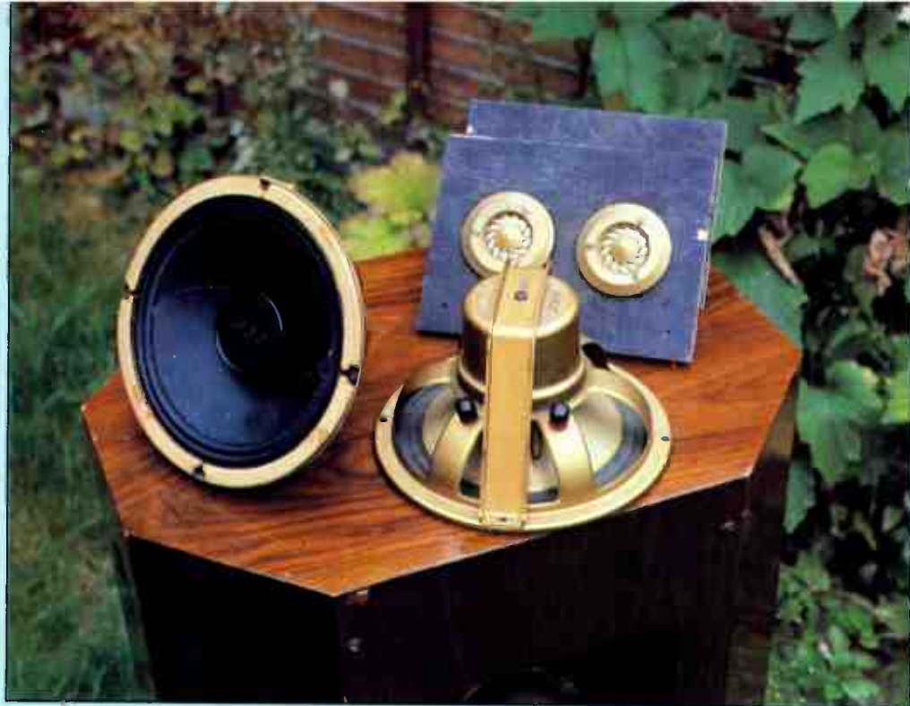
GEC produced metal cone loudspeakers back in the '50s, seen at the forefront here. Behind is the presence unit described in the article.
