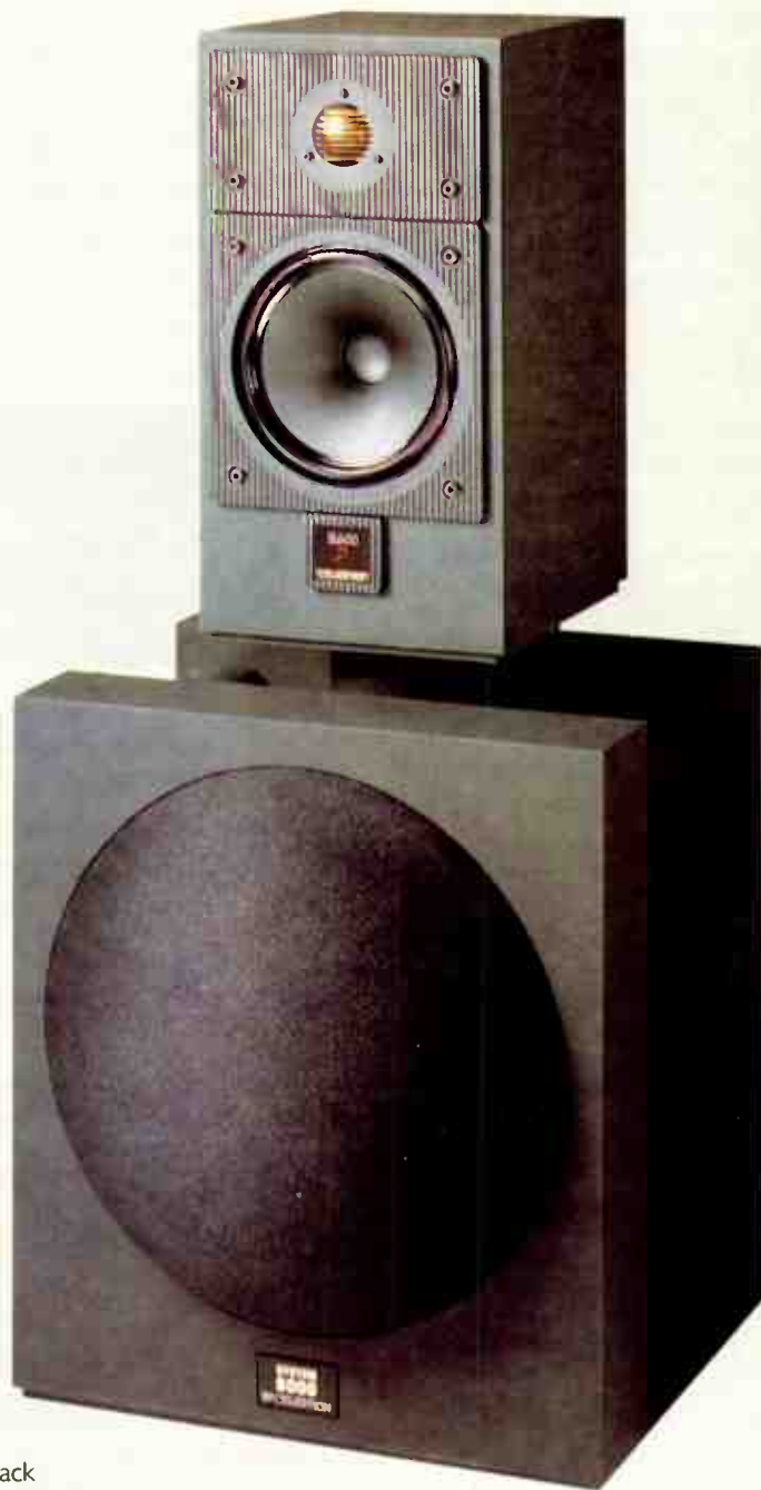
The Celestion SL-6000 double-dipole sub-woofer, supporting a Celestion SL600 box loudspeaker. Beneath the fabric dome lies a 12in paper cone bass unit. Each SL-6000 has two of them, one on the front baffle and one on the rear baffle. Because there is no box, there is no lower limit to the depth of bass it can produce; even 5Hz is possible.
