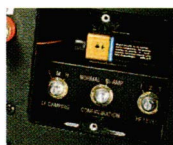
Crossover presets allow subtle adjustments to the frequency response.
