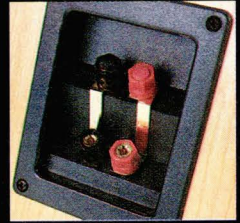
In the latest samples Royd has replaced the terminal joiners (above) with internal hardwiring for better single wire performance.
