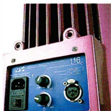
Volume and bass controls on the heavily heatsinked rear panel.
