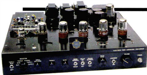
Pro-Logic II was developed using traditional valve technology, then transferred into a chip based processor.
