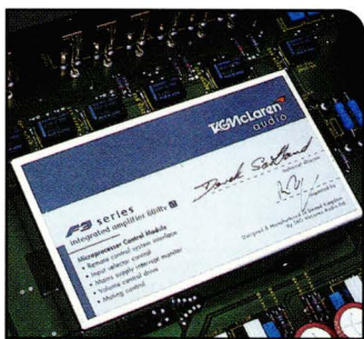
Signature electronics: the micro-processor 'brain' of the 60iRv amplifier.
