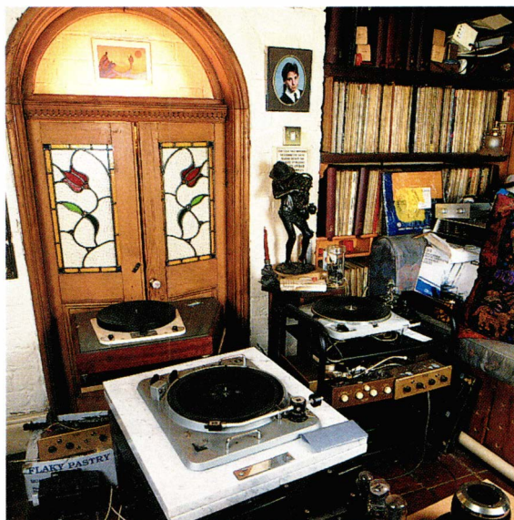
The mighty EMT atop a granite plinth outweighs a Garrard 301 (back) and another TD124 (right).
