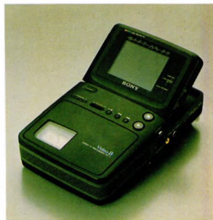
Top: The Alexander SE6 – a capable metal box. Below: A new must for the Filofax crowd, Sony's pocket-sized GV-8E has an LCD screen and plays Video 8 cassettes.
