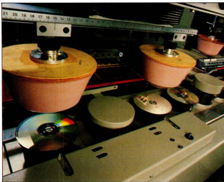
Above, rubber pads print the labels; Right, the complex equipment for lacquering CDs on the production line; Bottom (f page, the finished product – CD albums packed 25 to a box.
