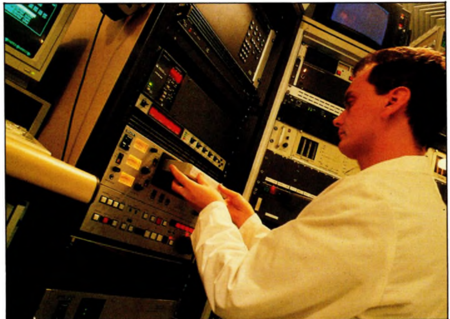
Top, a row of Sony and Ampex VTRs in the CDV mastering area. Below, a master tape for a 12in CDV being loaded.
