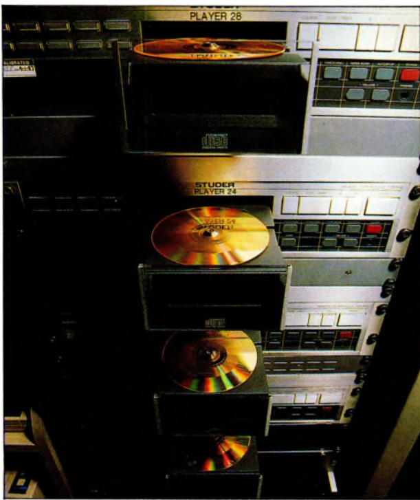
Left, 4 CDVs undergoing a 'content control' test; Above, preparation of the photo-sensitive glass substrate, under red lighting; Bottom of page, the continuous on-line metallising process for CDs
