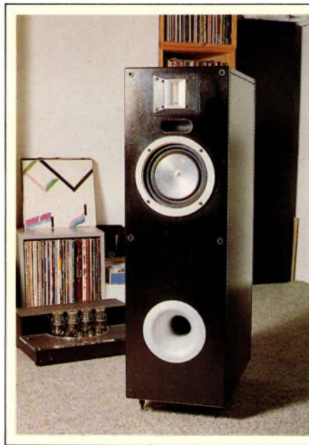
Townshend Glastonbury II. The aluminium cone bass/mid driver is used up to 7.6kHz, and the flared port tuned to match the driver's free-air resonance circa 27Hz. Crossover may be split; in normal use one of the links is a resistor to allow tweaking of the tweeter output level.
