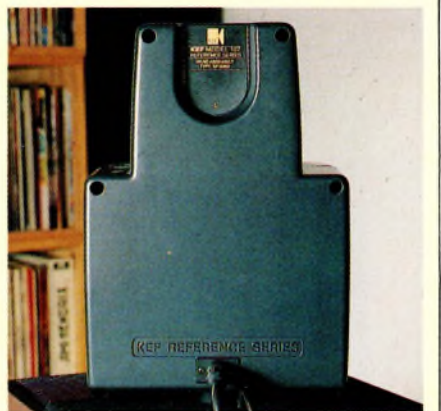
KEF107. Active bass equalisation in the form of the KUBE control box allows unprecedented flexibility in room/system matching. Top enclosure housing mid and treble units can be rotated to achieve precise stereo focusing, but results in it being non too rigid.
