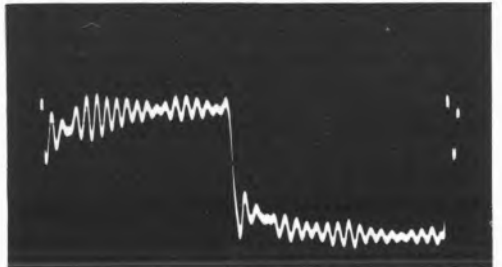
1 kHz squarewave (ignore ultrasonic cutter ringing)
