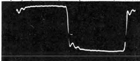
1kHz squarewave (ignore ultrasonic cutter ringing)
