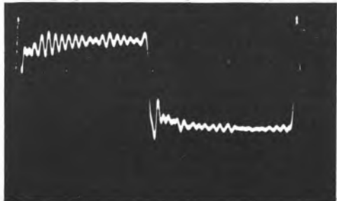
1kHz squarewave (ignore ultrasonic cutter ringing)
