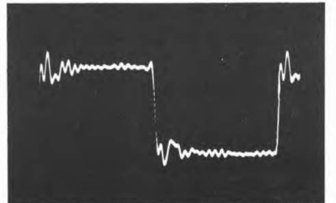
1kHz squarewave (ignore ultrasonic cutter ringing)
