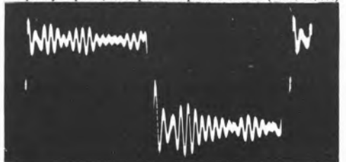
1kHz squarewave (ignore ultrasonic cutter ringing)
