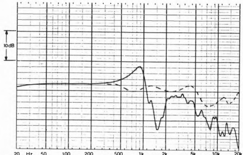
Frequency response, B&K4153 Artificial Ear, 'ideal' curve dotted.
