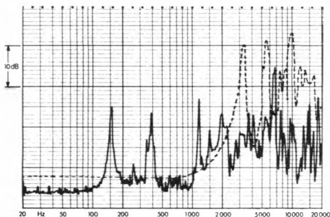
Arm resonances (compared to cartridge resonances, dotted).
