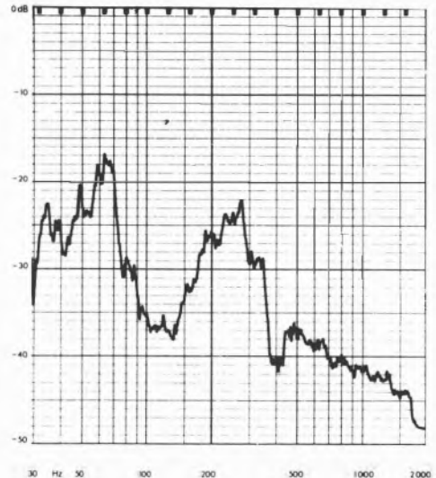
Acoustic breakthrough (microphony) of system (0dB = approx. 10 cm/s RMS, DIN rumble level, equivalent to loud music output from turntable).
