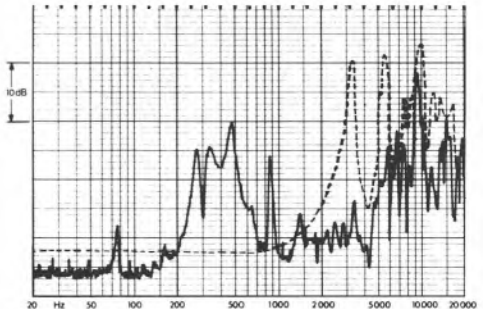
Arm resonances (compared to cartridge resonances, dotted).
