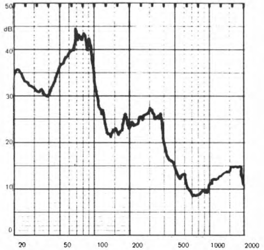
Indication of magnitude and frequency of arm resonances
