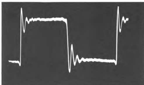
Photograph of squarewave characteristics at 1kHz illustrating transient performance.
