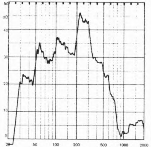
Indication of magnitude and frequency of arm resonances.
