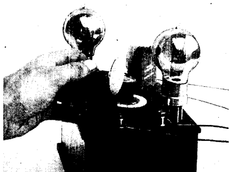
Fig. 16. Damping plates used with H.F. transformers vary the wave-length that is received
