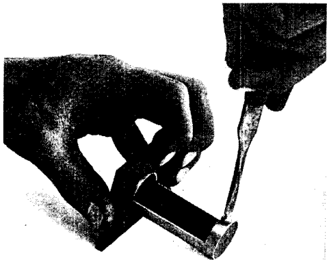
Fig. 7. Screwing the terminal to the fixed plate. Note the lock nut, which should be tightened
