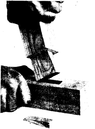
Fig. 6. This is a locked or dove-tailed mortise joint. The wedge locks the joint
