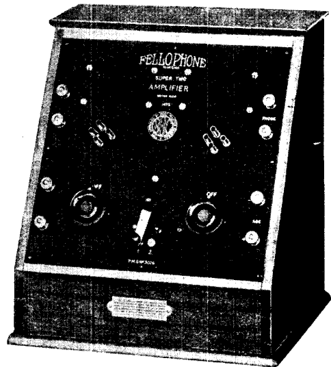
Fig. 3. This note magnifier also allows one or two valves to be used. The two lower knobs control the filament resistances
