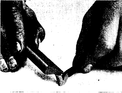
Fig. 2. How a lathe tool is sharpened with an oilstone slip is illustrated
