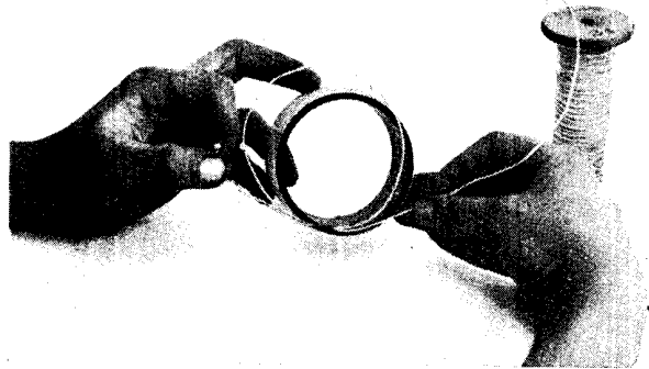
Fig. 9. Ends of the primary winding are twice threaded through a short length of sleeving to form a loop and then pulled tight
