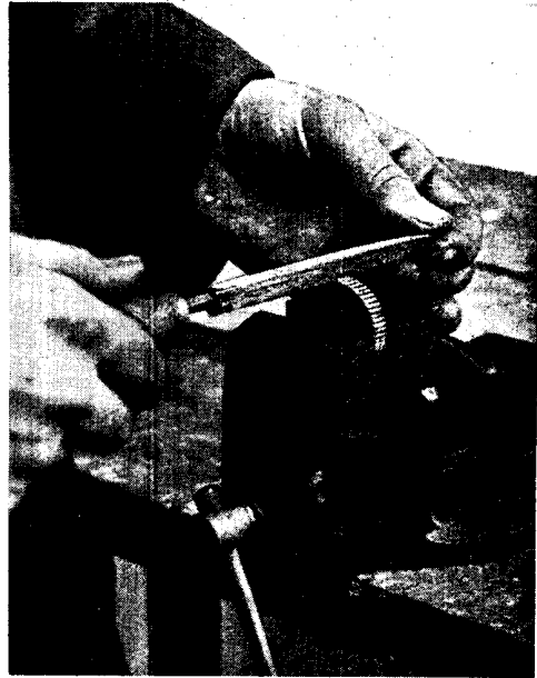
SERRATING THE RIM OF A KNOB
