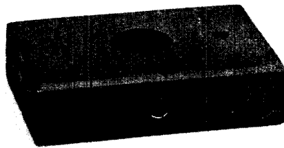
Fig. 11. An ebonite block forms the foundation of the jack. Note the position of holes, also chamfered edges
