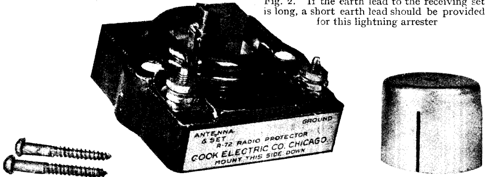
Fig. 3. With the cap removed, the interior of the metal-carbon gap type of lightning arrester is seen in this photograph, and the two elements forming the gap are clearly visible. The base is of porcelain, and screw holes are provided for attachment to a permanent structure. One of the terminals is connected to earth and the other to the aerial
