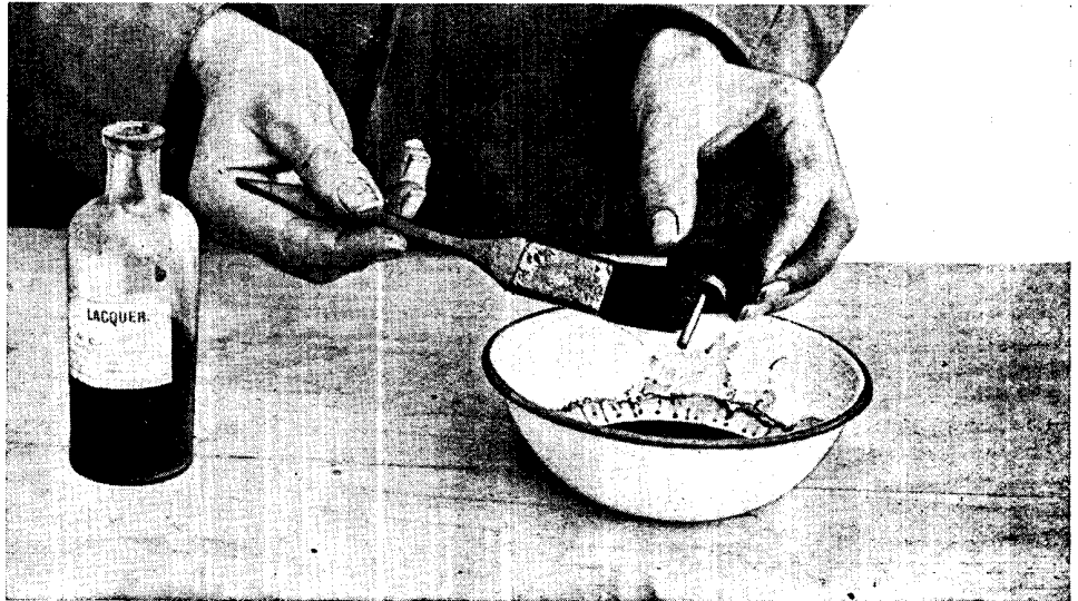
Fig. 4. Lacquer is placed in an open vessel and applied to the object being treated with a soft brush. The actual part being lacquered must not be touched by hand
