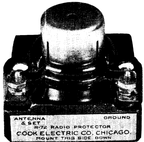
Fig. 2. If the earth lead to the receiving set is long, a short earth lead should be provided for this lightning arrester
