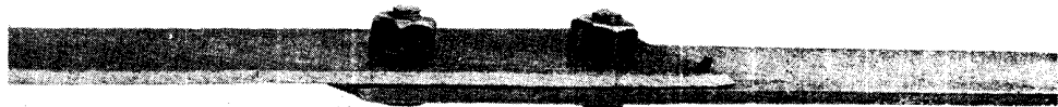
Fig. 12. Thick metal plates which cannot be folded and hammered, as in Fig. 11, may be overlapped and riveted, or connected by bolts and nuts, provided good clean contact is made and the plates are very tightly joined
