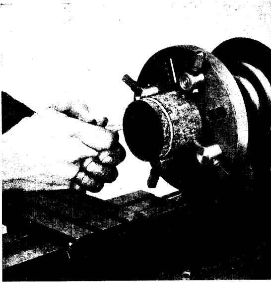
Fig. 8. Tracing up is being carried out with the aid of a piece of chalk
