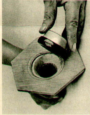
Fig. 10. Hollowed block for receiver of loud speaker
