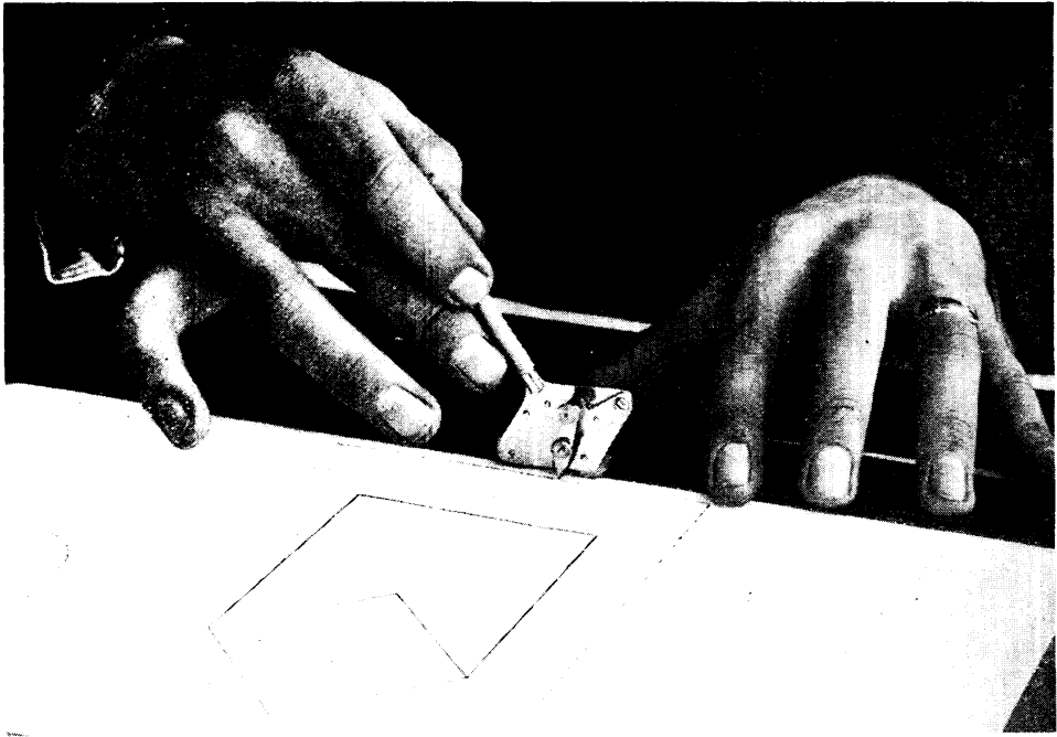
Fig. 5. Dotted lines in a finished drawing are essentially required to be neatly made. Unaided, considerable skill and patience would be required of the draughtsman, but with the automatic dotting pen much time is saved and the dots are evenly spaced!
