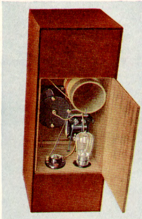
Fig. 110. Second view of back of cabinet, showing valve in place and stable crystal detector
