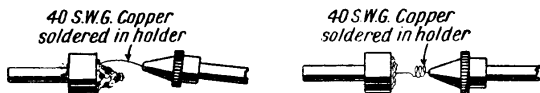
Fig. 52. Searching the crystal can be carried out by drawing the cat's-whisker across the surface and by rotating the crystal cup. For flat crystals the fine adjustment is used to alter the tension of the cat's-whisker point upon the crystal without shifting its position
