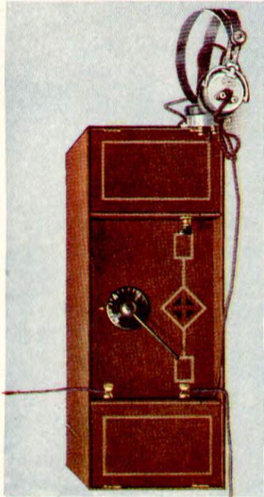
Fig. 100. The self-contained set complete and connected to aerial and earth ready for use
