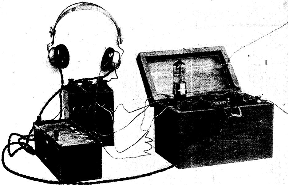
Fig. 84. In the telephone recess of the original crystal receiver is fitted a low-frequency transformer and a panel on which is mounted a valve and filament resistance. The complete set is here shown joined up with the low-tension accumulator and a high-tension battery with wander plugs. The crystal detector circuit remains unchanged
