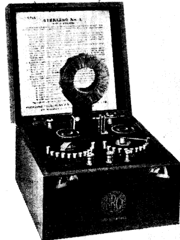
Fig. 5. Plug-in loading coils may be used in this variety of receiver Courtesy Sterling Telephone and Electric Co.
