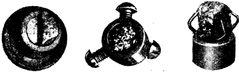
Fig. 4. Three methods of setting crystals in their cups are shown. Left is a crystal in plastic metal, centre the screw-grip method, and right is a cup with four spring claws
