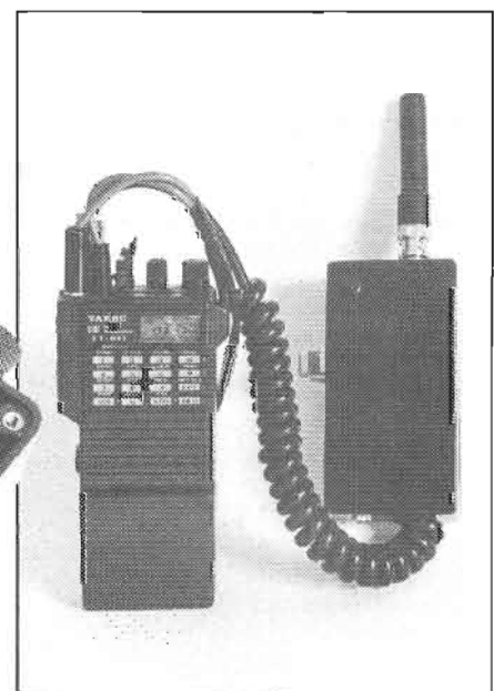
Projects – Add-on BFO unit (centre) and a speaker mic (below)
