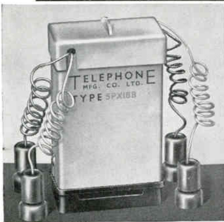
The Type 5PX Carpenter Polarised Relay is fitted with platinum contacts to reduce thermal noise, and has flying contact leads to reduce "pick-up" in contact circuit due to the coil. DIMENSIONS: Height 2.5 in. Width 1.6 in. Depth 0.8 in. Approx. weight 4.8 oz.
