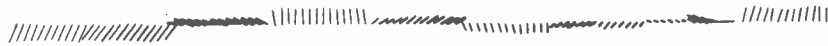
Fig. 1. A typical record obtained with the automatic apparatus. The vectors represent the phase and amplitude of the cross-modulation at frequencies of 60, 120, 300, 500, 700, 1,000, 1,250, 1,500 and 2,000 c/s.
