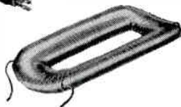
3 Field Coil for motor car dynamo wound with 280 turns of .030 inch enamelled wire.
