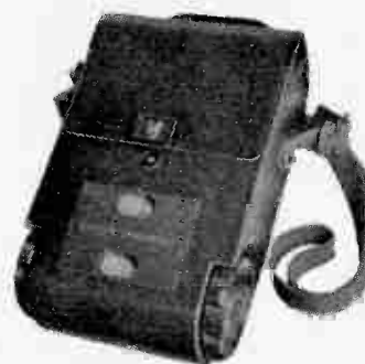
Fairey photo-electric safety ohmmeter. The selenium cell is concealed by a hinged cover which is lifted in use
