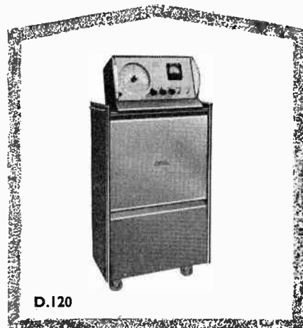
Frequency Range : 10-10,000 c/s. in 3 ranges. Calibration accuracy : \pm 2\% . Power output : 120 watts into 10 ohms at unity power factor.
