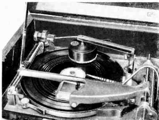
Microgroove recorder used in radiogramophones by M.S.S.
