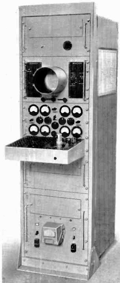
Cinema-Television universal valve tester in which any desired valve characteristics can be displayed on a calibrated c.r. tube.
