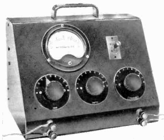
British Physical Laboratories precision frequency meter, 10-110 c/s.
