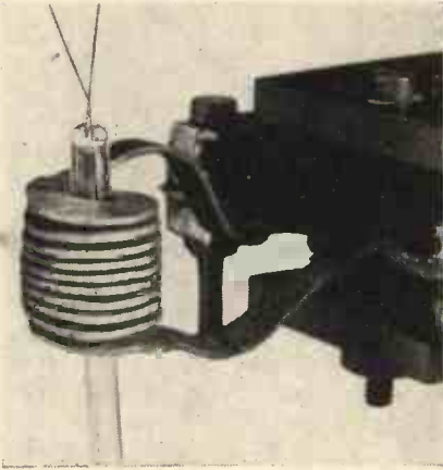
Close-up of heating coil, gettering valve on pump.
