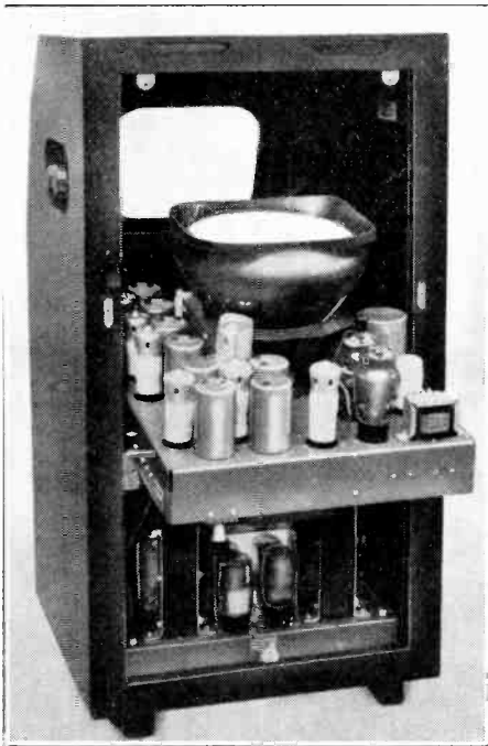
The interior of the Murphy T56 television receiver showing the chassis tilted back for inspection.
