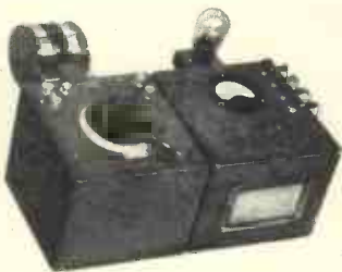
The wavemeter used for Absorption Measurements by strapping Units R800 and R800.A.
