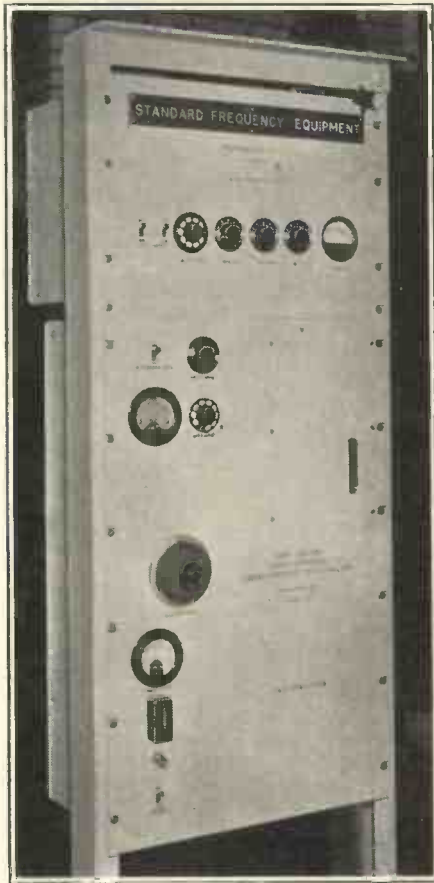
Fig. 6.—Sullivan Heterodyne generator for use with the apparatus shown in Fig. 5.
