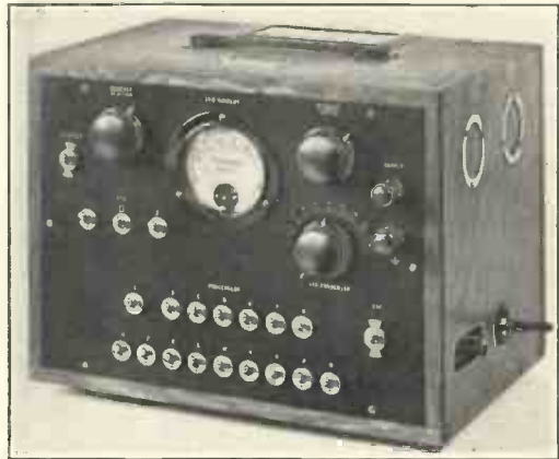
Standard Telephones A.C. mains-operated oscillator for audio-frequency tests
