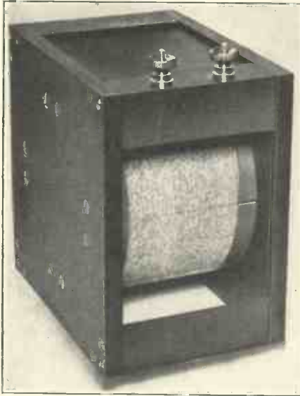
Fig. 1.—Sullivan-Griffiths thermal compensated inductance; single layer type.
