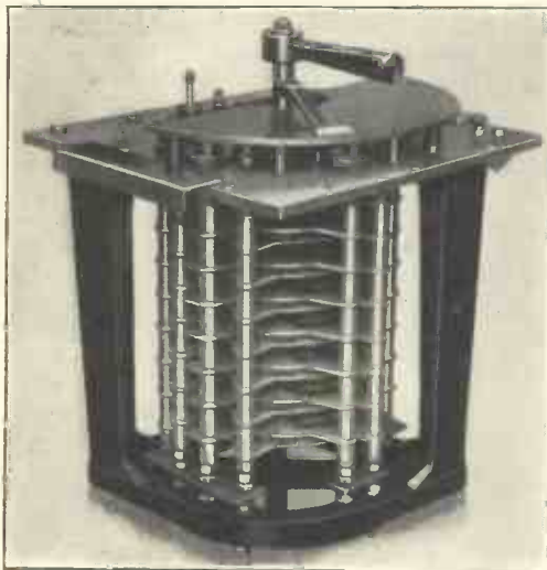
Fig. 3.—Sullivan-Griffiths series-complementary dielectric gap variable condenser.
