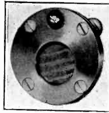
Copper oxide photo electric cell. A new product shown at the Exhibition.
