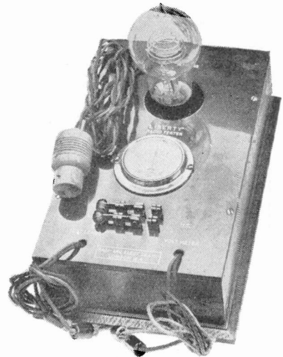
The Liberty testing set for voltage measurements, continuity and insulation tests.
