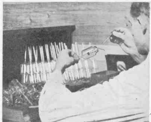
Fig. 3.—Welding the foot into the bulb.
