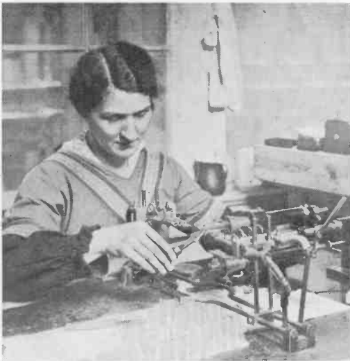
Fig. 1.—Turning the glass feet on a "lathe."
