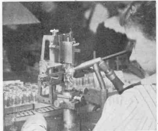
Fig. 2.—A machine which forms and welds the electrodes.
