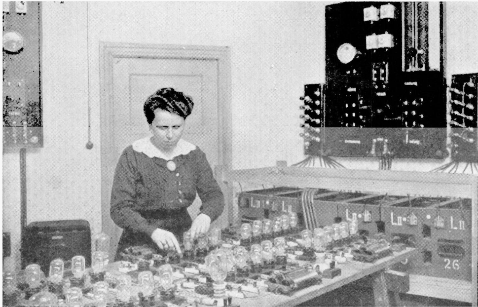
Fig. 12.—Ageing test of valves subjected to abnormal anode voltages.
