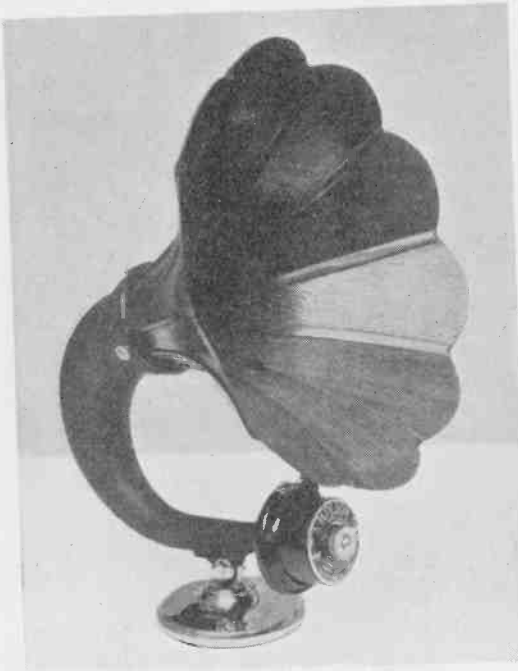
In the new Amplion the metal is welded and pressed and a wooden horn is used to prevent resonance.
