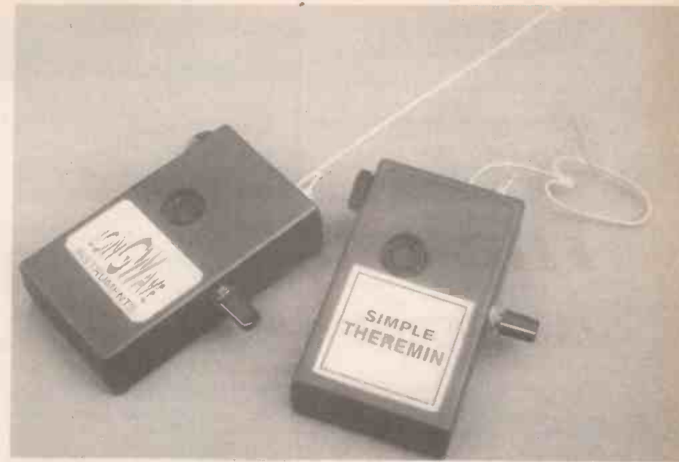
Two versions of the Simple Theremin, only the Pitch conductor shape has been changed.
