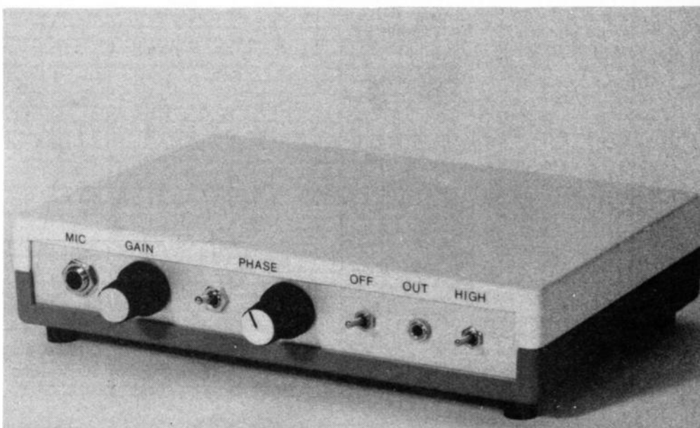
The completed Experimental Noise Cancelling Unit showing front panel lettering, using the Phase Shifter board.
