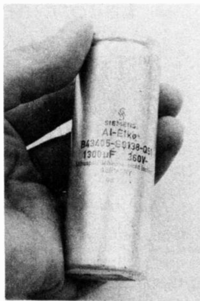
A high voltage capacitor can store a dangerous charge.
