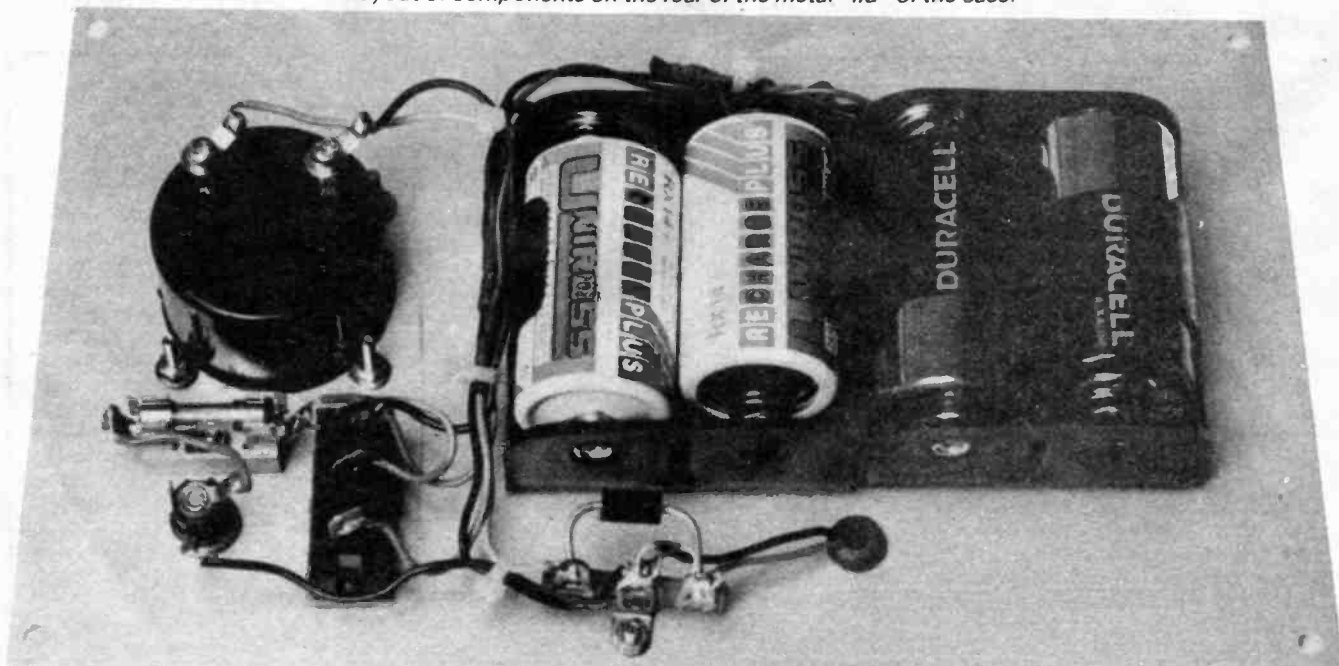
Fig. 2. Interwiring between components. Tag 2 is also used for bolting the strip on the metal panel.
