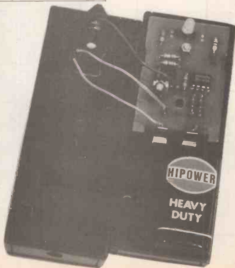
Fig. 2. P.C.B. layout and wiring for the Quicktest.
