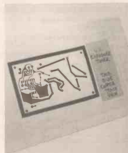
The artwork is turned over and clearly labelled "Copper Track View Side" – this is your first sight of the actual copper foil pattern which will be etched into your p.c.b.!
