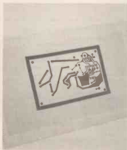
The completed artwork on the light box—the precision 0.1in. matrix grid is also visible. This view is actually equivalent to seeing the copper track pattern "through" the board from the component side.
