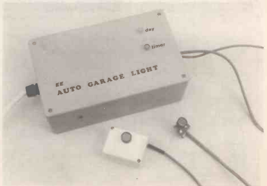
The completed garage light controller showing the Day/Night and Headlight sensors.
