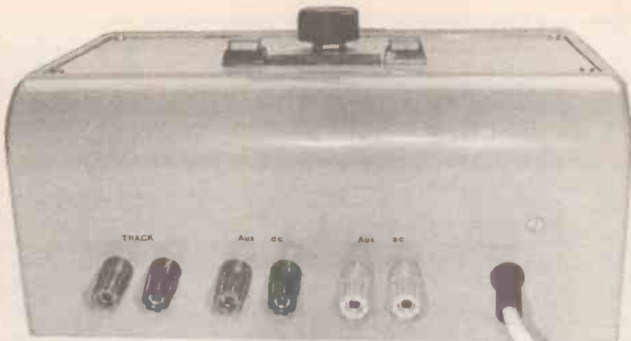
Rear view of the case showing the three groups of output sockets/terminals.
