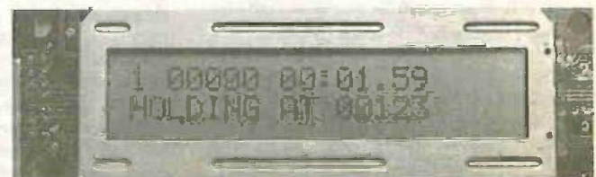
Photo 4. Typical I.C.D. display when first switching power on after a previous batch of data has been sampled.
