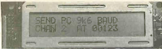
Photo 5. Typical l.c.d. screen during data transfer to PC, the baud rate is confirmed as 9600.
