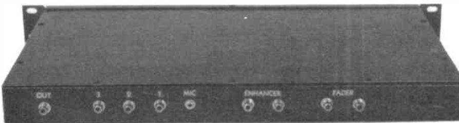
The Audio Mixer input and output sockets are mounted on the rear panel of the case.
