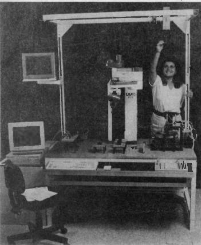
Demonstration setup the RTX robot arm from UMI with its new workcell, together with an "overhead" vision system.
