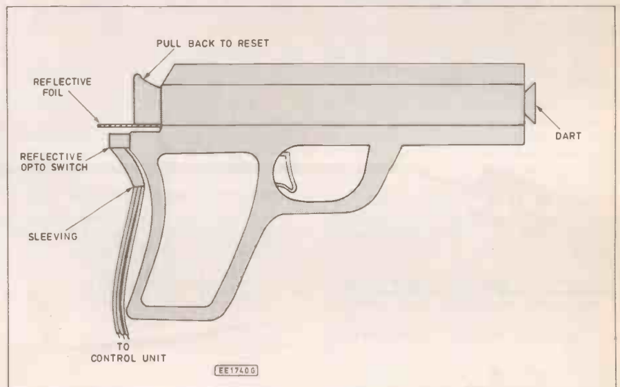
Fig. 3. Mounting the opto-switch on the gun.
