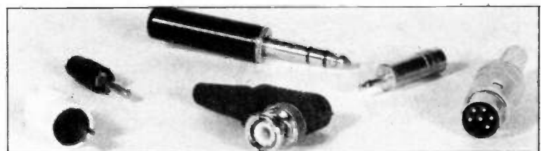
A plug assortment (2 pin DIN, 4mm, stereo jack [rear], BCN [front], 2.5mm jack and 6 way DIN).
